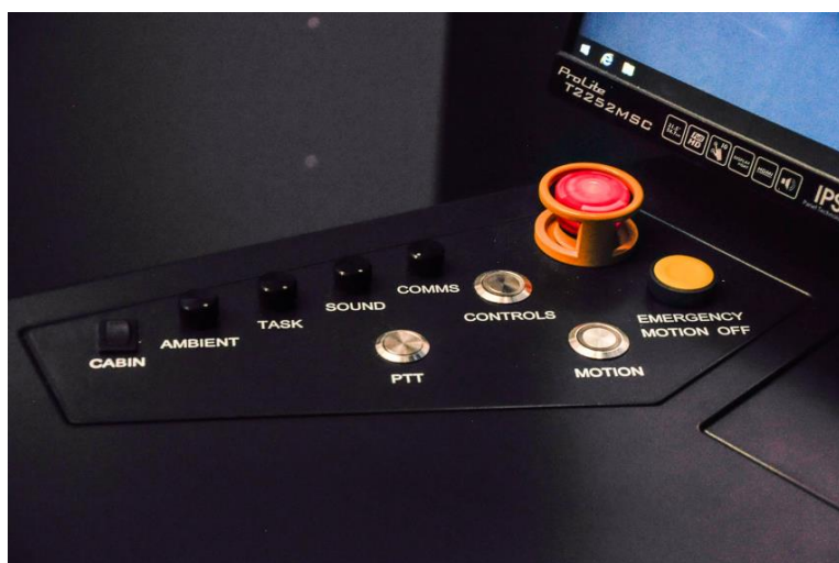
Fig. 2: IOS Control Panel
