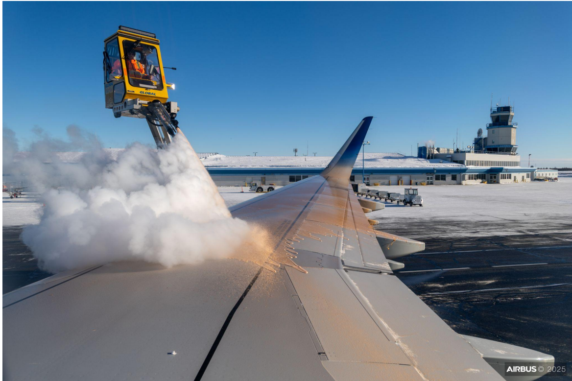
Treatment with Type I Fluid
