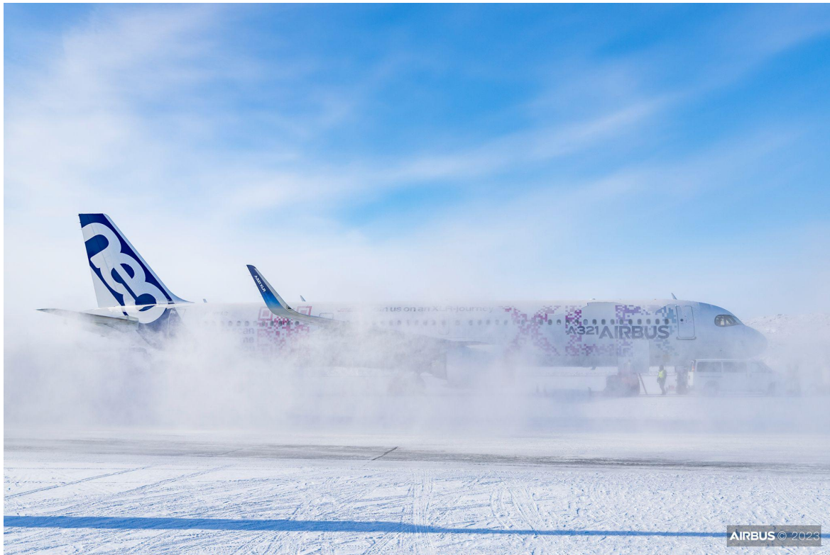
Possible Contamination due to Wind on the Ramp
